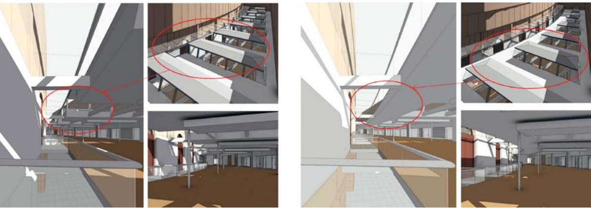
Figure 9 – Roof skylight options A (left) and B (right). Source: the Author.
